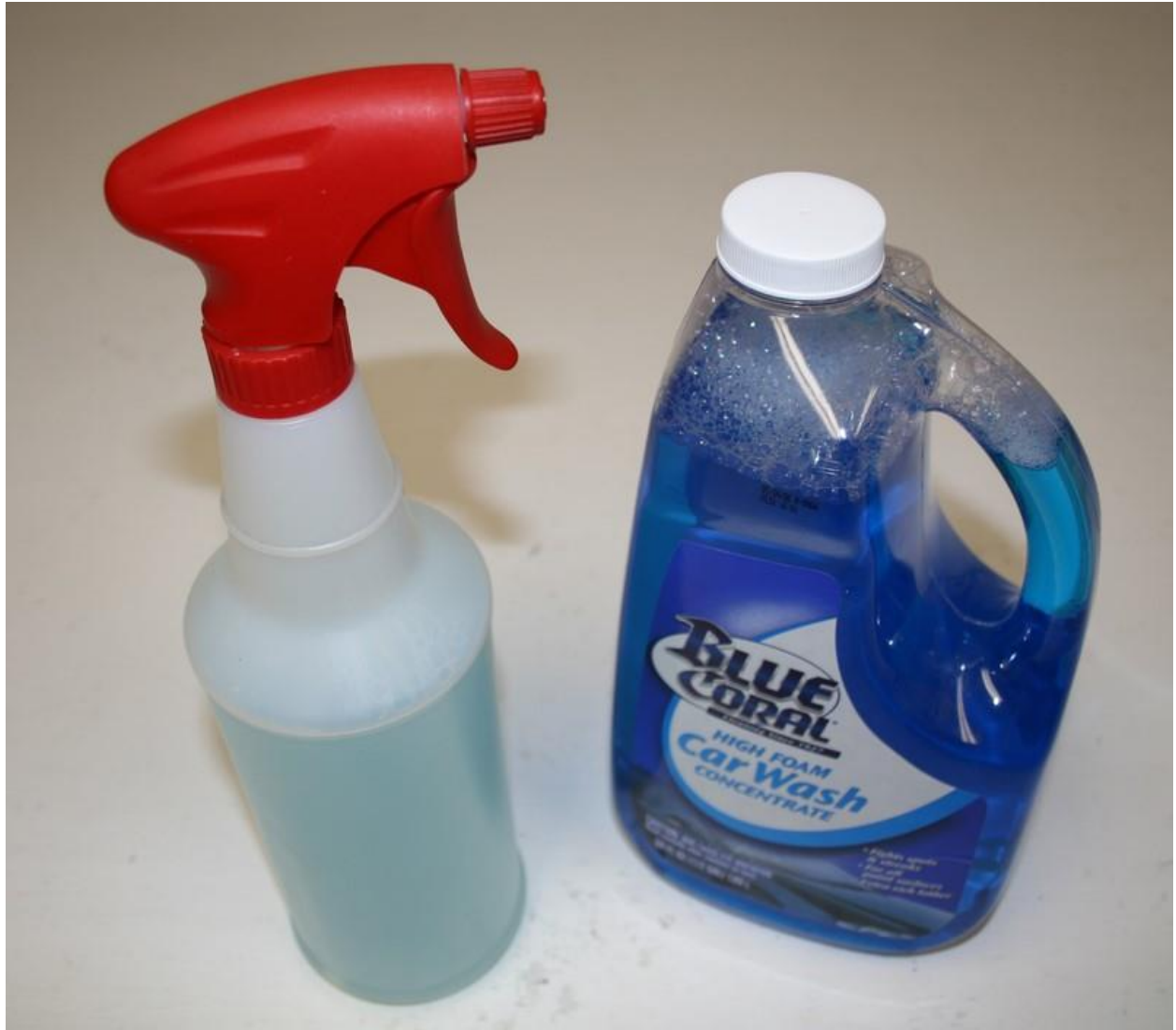
Photo 16 - After running out of the Meguiar's Quick Detailer, we mixed a cap full of Blue Coral car wash with water in a spray bottle which will now act as our surface lubricant.
