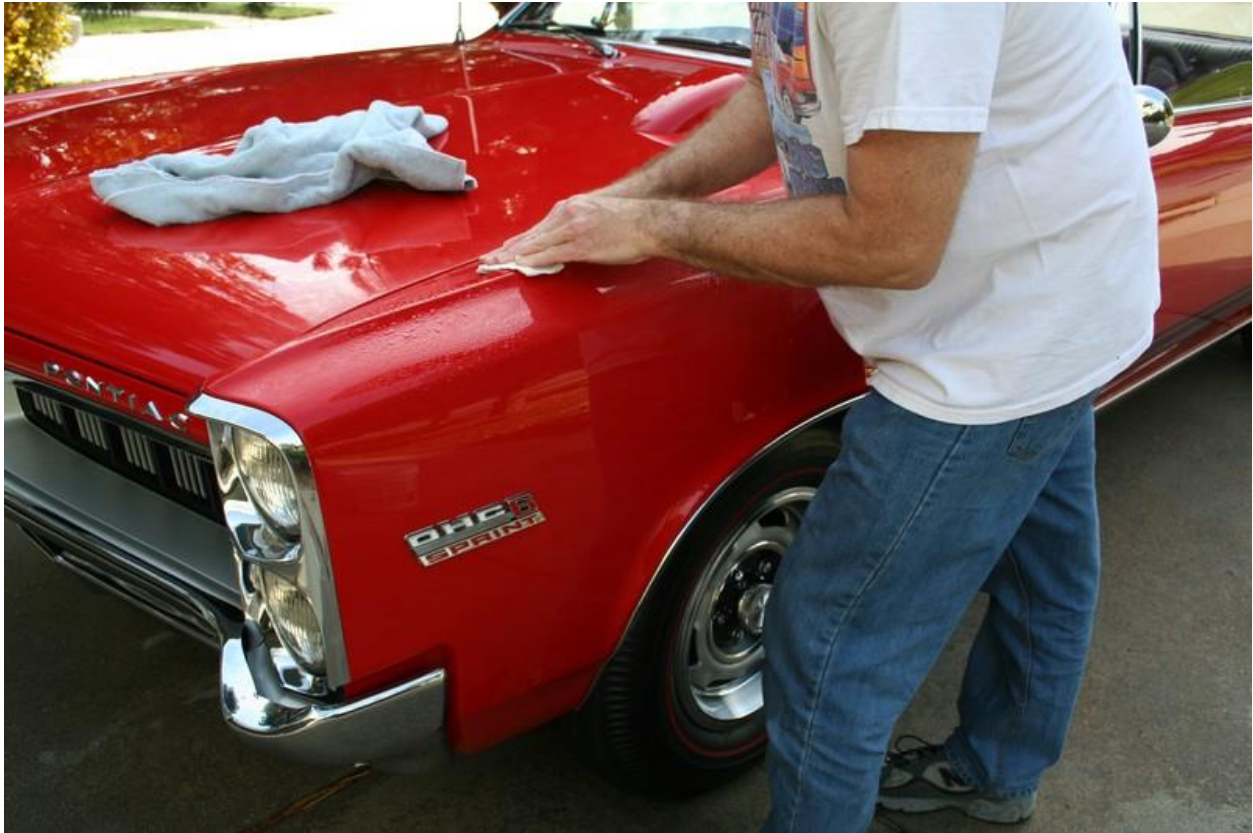
Photo 15 - As one side of our clay bar became soiled we flipped to the other side and kneaded and refolded the clay as required to keep a side clean.
