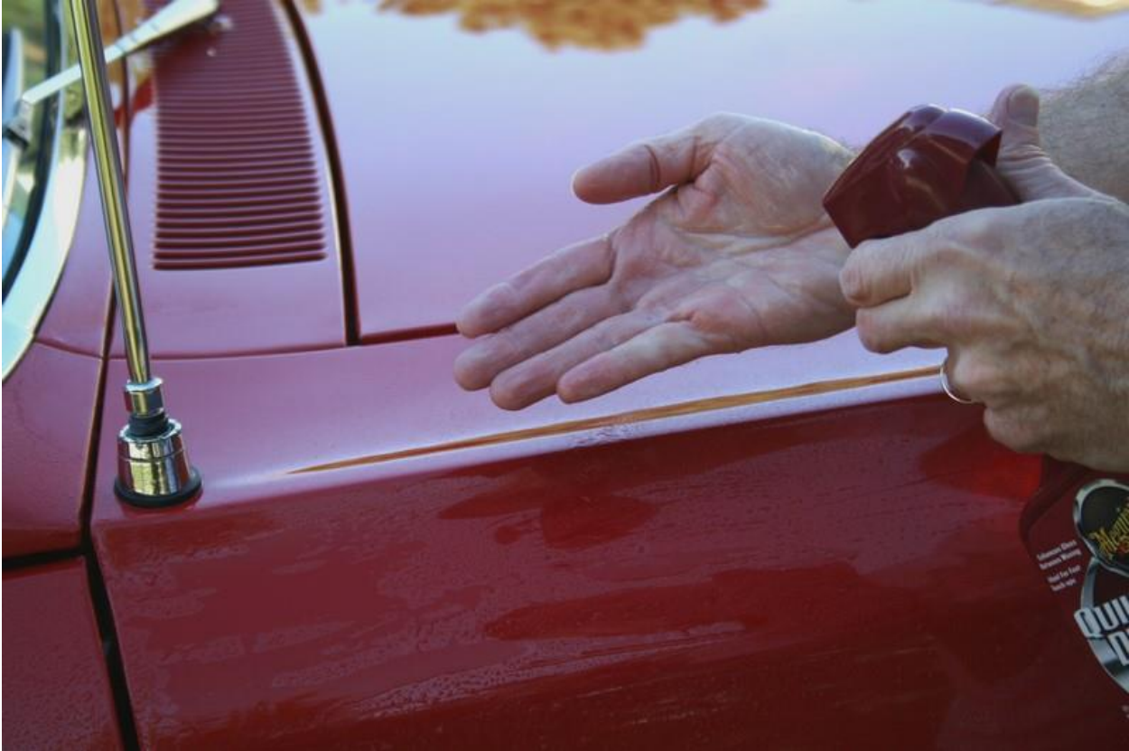
Photo 10 - We also treated our hands with the lubricant to keep the clay from sticking to them and coming apart as we worked.
