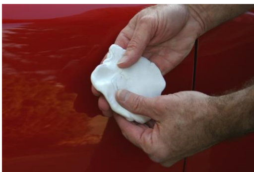
Photo 15 - As one side of our clay bar became soiled we flipped to the other side and kneaded and refolded the clay as required to keep a side clean.
