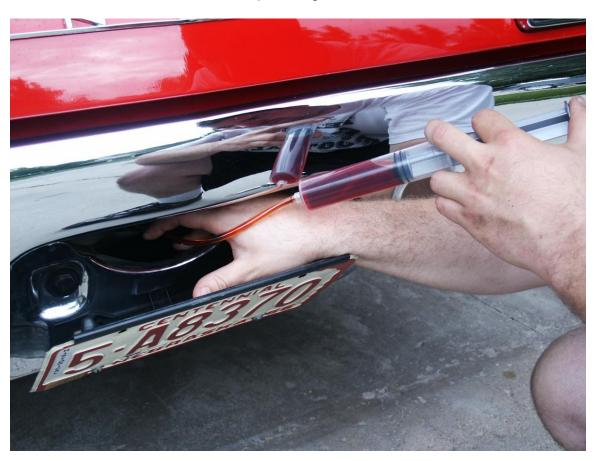
Step 5b - We used a common syringe to add the fuel stabilizer to the rear license plate location. Start the engine and let it run so that the fuel stabilizer can work its way through the entire fuel system.
