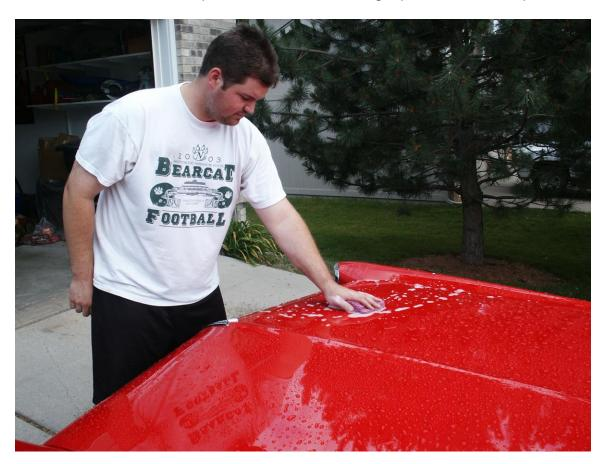
Step 2 - Apply a fresh new coat of wax and buff for additional protection. Applying the wax by hand also is fine. The new wax coat will help prevent chaffing of the paint while under a car cover, thereby helping to prolong your car's finish.
