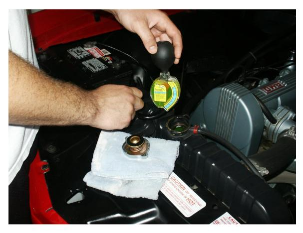
Step 7b - Almost all auto parts stores now have 50/50 premixed coolant. Start and run the engine one last time so all added fluids can circulate fully, and turn on the air conditioning (if equipped) to lubricate the compressor's seals.
