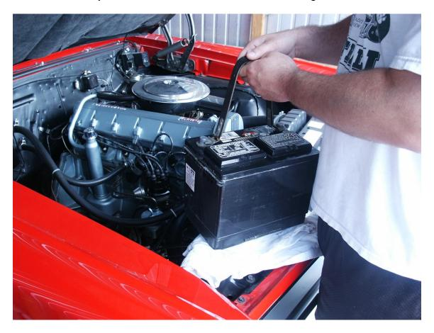
Step 11 - Never store a battery directly on concrete which will cause the battery to discharge over time. Setting it on wood blocks or a lower shelf is a good alternative. The use of a small battery charger, such as Deltran's Battery Tender Plus, can maintain the battery's charge during storage automatically.
